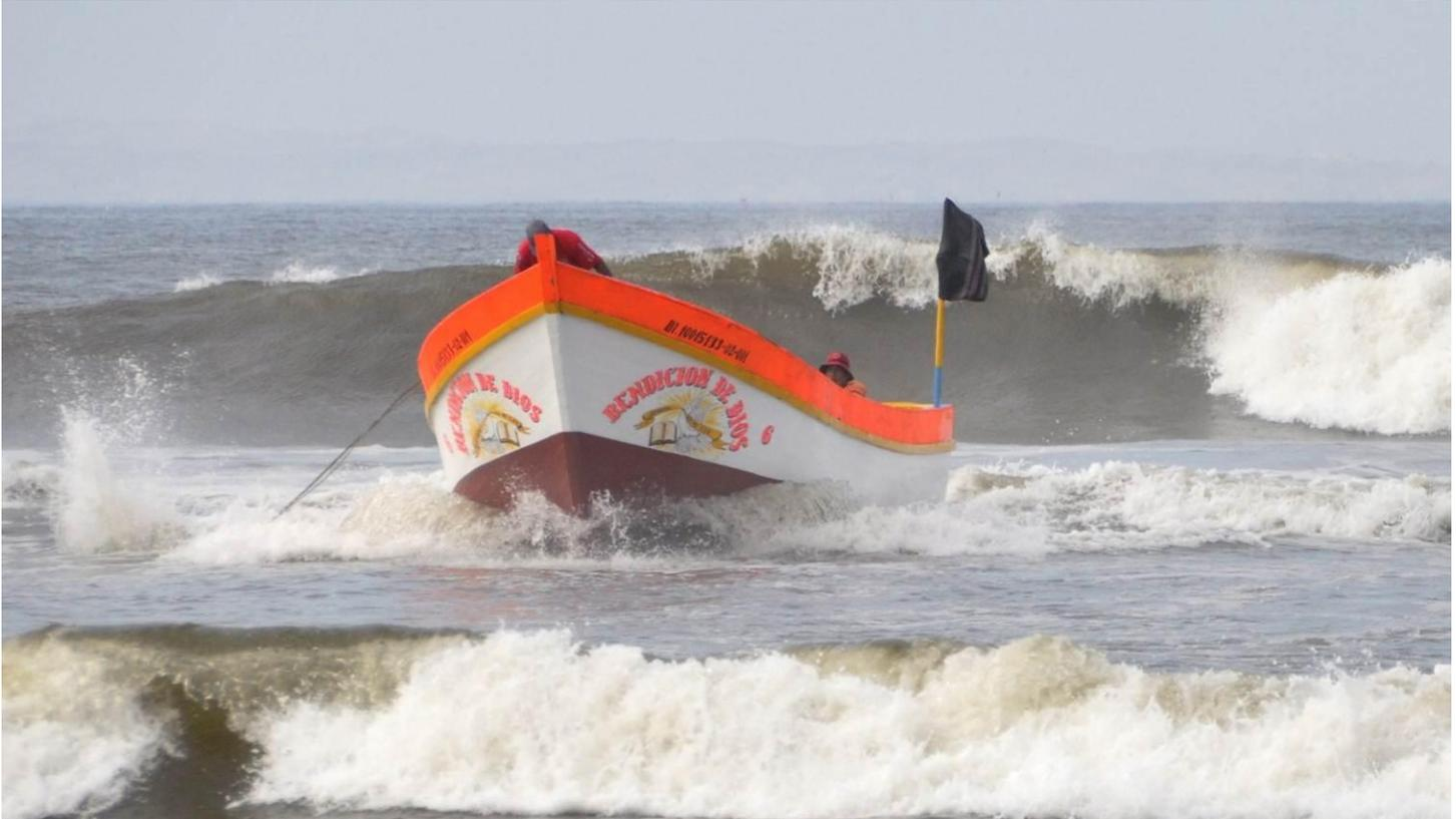
The boat rides the waves then anchors and swings broadside to allow loading – offloading on the beach
