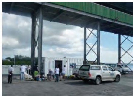
Pictures 12 and 13: The mobile lab used by the Mauritius Oceanographic Institute in collaboration with the IOI-SA for the PBBS in Port Louis is built into a container that can be moved to the quayside during a survey. It has all the electrical and plumbing adaptations needed and contains adequate storage, microscope, computing and sorting facilities.
